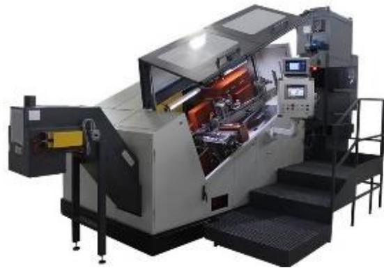
The Thread rollers issued with Double Starter Units are equipped with the **“M-Group”** which it provides the motorization of the drive unit and slide body position for quick and accurate control of the die match. All the adjustments are stored for each parts and can be recall to proceed with the automatic set up of the machine.
