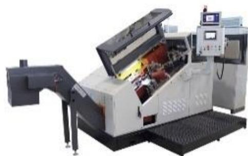
the vibratory feeder have the motorization of the height positioning to facilitate the adjustment according the length of the parts. The machine comes with a **vibratory feeder** as standard feeding system included in the sound proof enclosure.
